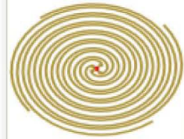
4-arm Archimedes spiral antenna
