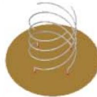
Open-ended quadrifilar helix (O-C QHA)
