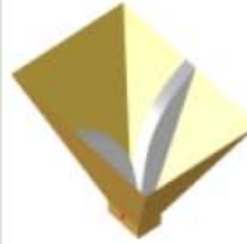
Ridged pyramidal horn
