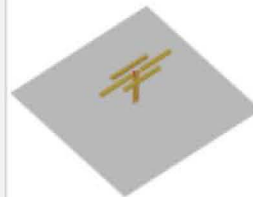
Open sleeve dipole
