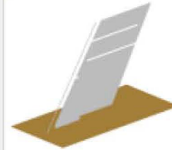
Planar blade antenna
