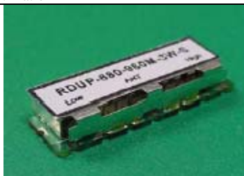
Duplexer, GSM Band 880-960MHz SMT . Bandwidth of 25 MHz, in band insertion loss of 3.5dB and rejection of 50dB. a cost effective solution.
