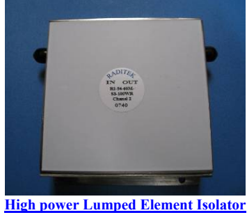
High power Lumped Element Isolator LL1 for DIGITAL TV Band 1, 49-88 MHz, SMA Connectors, 100 Watts 6 MHz Bandwidth. Also LL2 Band 3.
