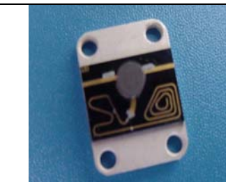
Microstrip Isolators and Circulators to 150GHz. Thin Film, Gold on Copper, many form factors, With and without Carrier
