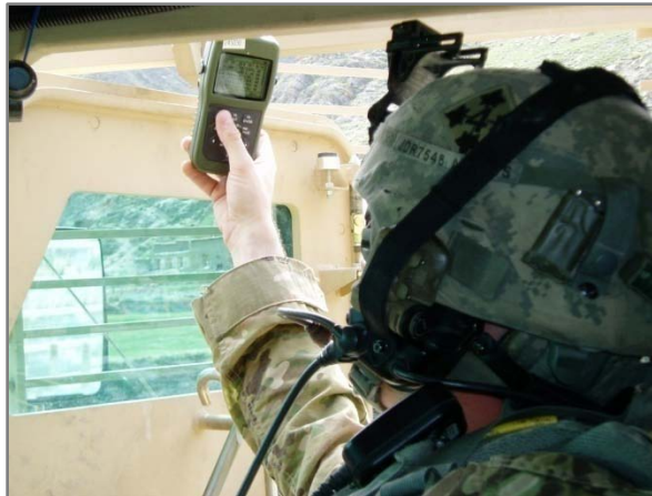
Figure 1. US Soldier Holding DAGR Through an Open Door to Acquire GPS Signal. Practices Such as This Dramatically Reduce Survivability Against a Range of Threats
