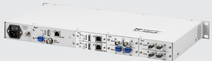
rear view 8029HEPTA Industry with 3 mutually independent NTP time server, 2 x IRIG-B analogue (BNC connector), 2 x IRIG-B digital (plug-in screw terminal) as well as 2 x DCF77 pulse and 2 x cyclic pulses (fiber optic in each case)
