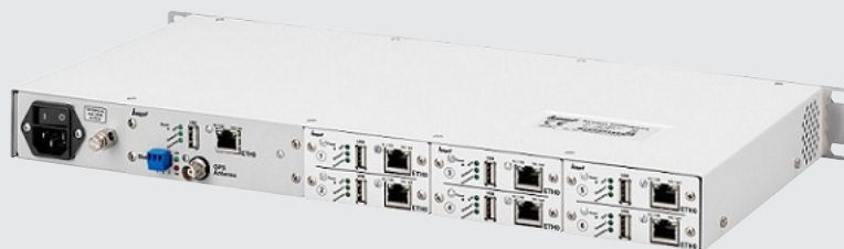
rear view 8029HEPTA DataCenter with a total of 7 mutually independent NTP time server
